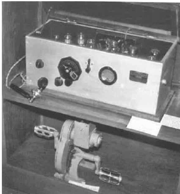
No 36 set with pedal generator on the shelf below it.
