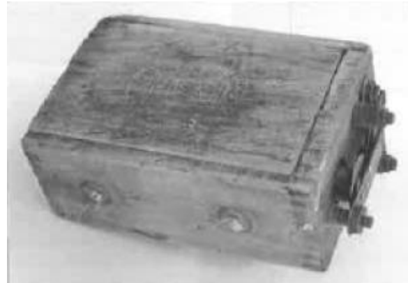
Model T coil as used to power the Hermannsburg and Arltunga experimental radio stations.
