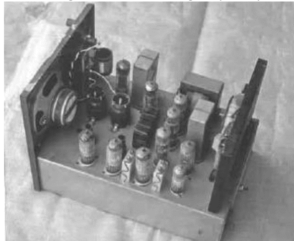
Internal new School of the Air transceiver type 505A
