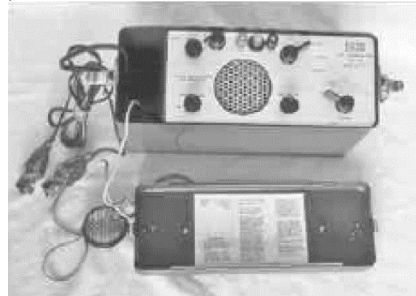
Elico 6104 (Codan), portable "Lunch Box" high frequency (HF) transceiver complete.
