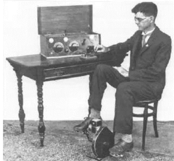
Alf Traeger posing with the original “baby” pedal radio transceiver.
