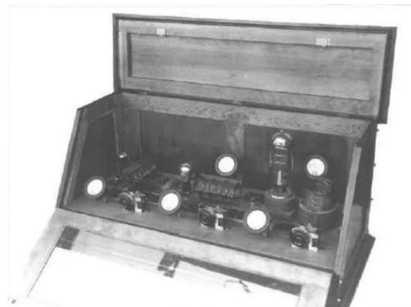
First Cloncurry base station transmitter. This was a 3 valve unit rated at 50 watts. It used grid modulation to provide voice transmission.
