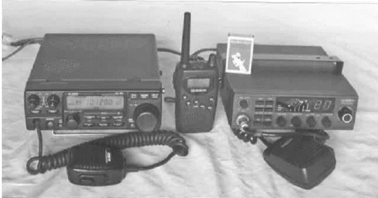
Left to right A high frequency (HF) multi mode (AM, FM, CW and SSB) 100 watt PEP amateur radio transceiver, a 0.5 watt 40 channel hand held UHF, FM, CB transceiver and 27Mhz AM/SSB CB transceiver.
