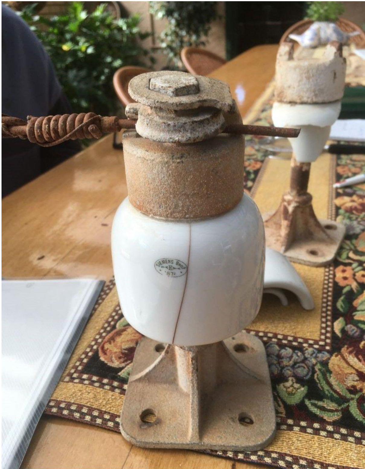
Siemens Bros 1876? insulator and locking device on W A wooden posts and join in wire
