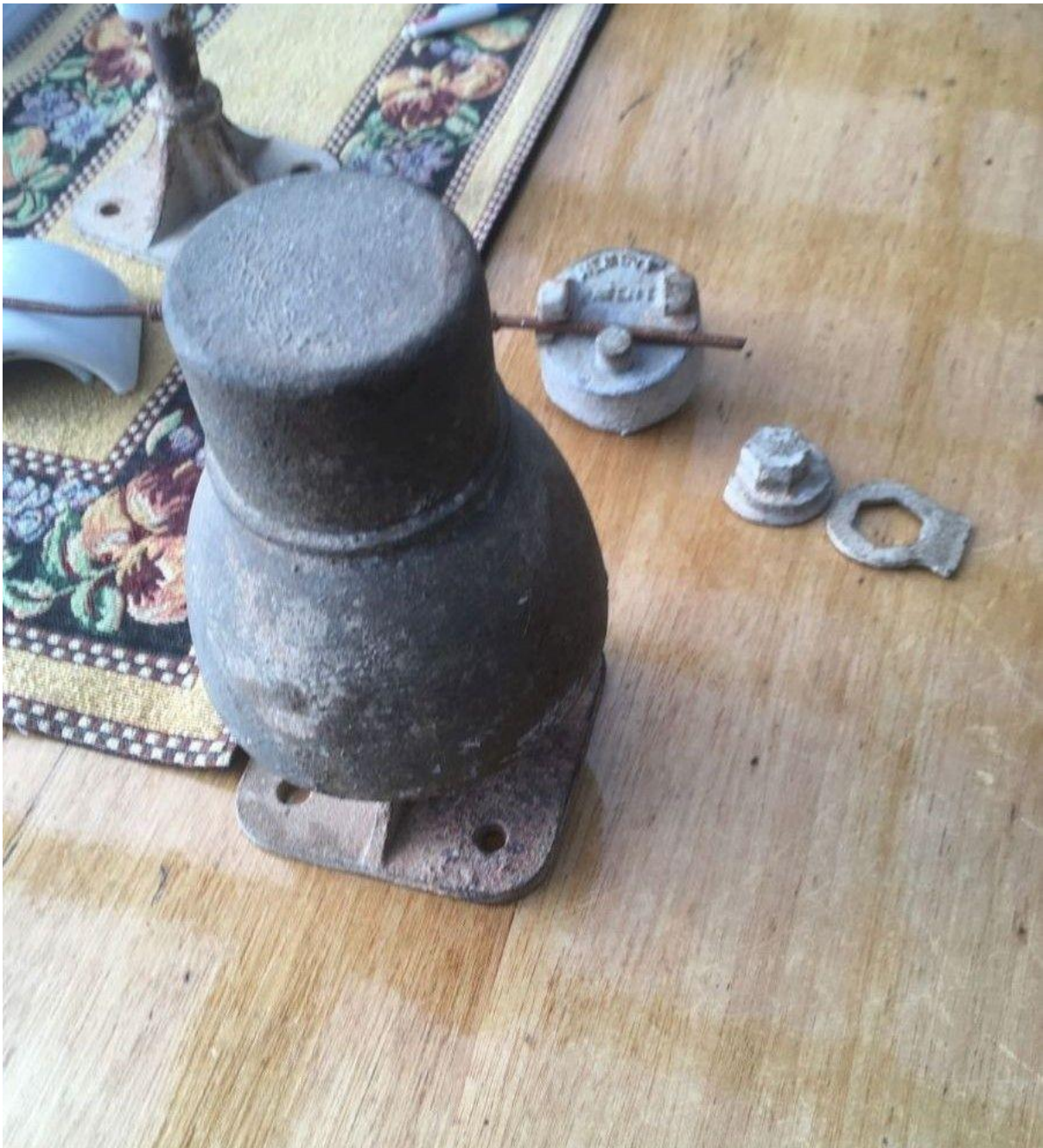
Metal insulator & Siemen's insulator top with cam nut and spanner (at back)
