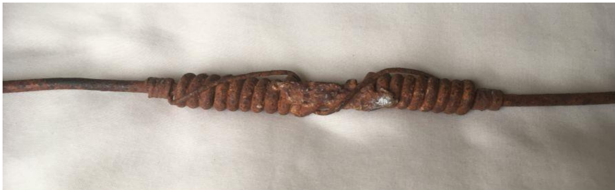
Telegraph wire join soldered centre & both ends
